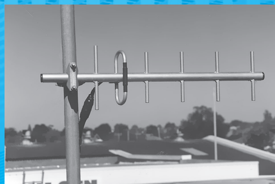
9 Element with 9 dBd gain
