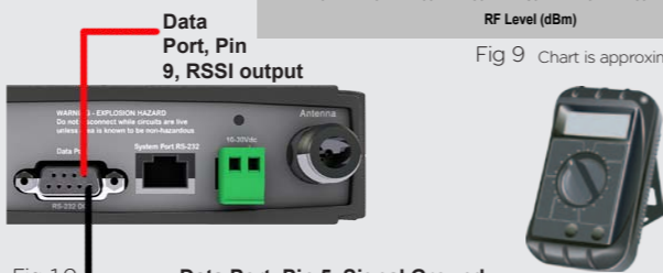
Fig 10 Data Port, Pin 5, Signal Ground
